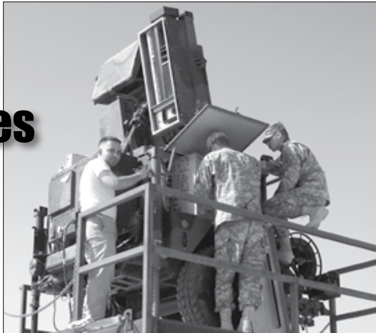
Steve Farthing (left), Raytheon Sentinel field service representative, SPC Doug Tindall (center) and PFC John Geoffroy, Sentinel operators of C Company, Special Troops Battalion (C/STB), 82nd Airborne Division (82 Abn Div), perform maintenance on the Sentinel radar at Bagram Airfield, Afghanistan. (Photo by 1LT James Wagner, C/STB, 82 Abn Div)
