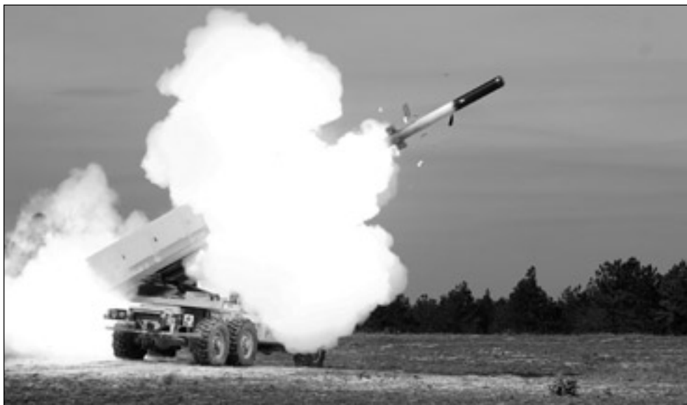
A reduced-range practice rocket leaves the tube of a HIMARS during 2-27 FAR training and qualifying at Fort Bragg, North Carolina. (Photo by GMG3 Jonathan Kammen, US Navy, Retired)
