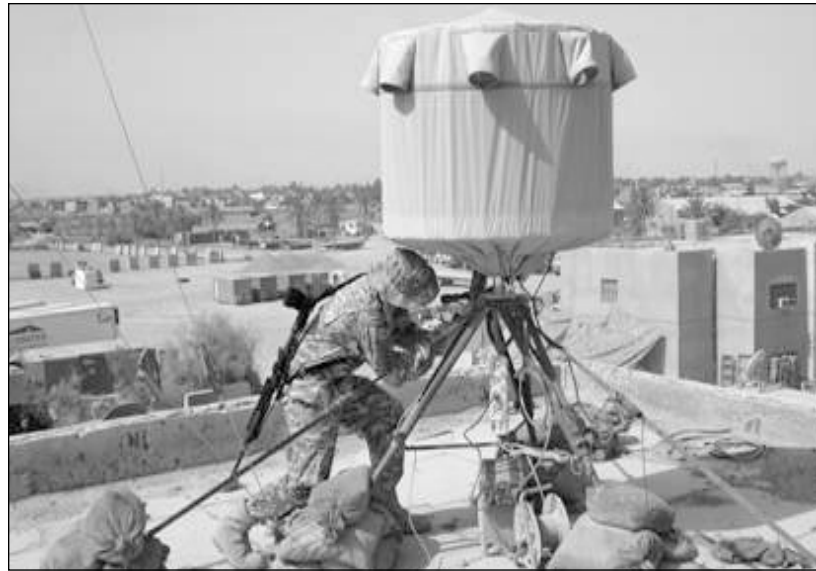
SSG Sean Ciardi, 5th Battalion, 5th Air Defense Artillery (5-5 ADA), bore sights a Lightweight Countermortar Radar (LCMR) at Combat Outpost Corregidor, Iraq. (Photo by 1LT Michael Ratcliff, 5-5 ADA)
