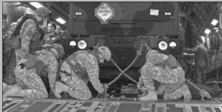
Members of Battery C, 1st Battalion, 158th Field Artillery, Oklahoma Army National Guard (OKARNG), chain down a High-Mobility Artillery Rocket System (HIMARS) launcher in the "belly" of a US Air Force C-17 cargo aircraft on 25 April. (Photo by CPT Geoffrey J. Legler, OKARNG Public Affairs)
