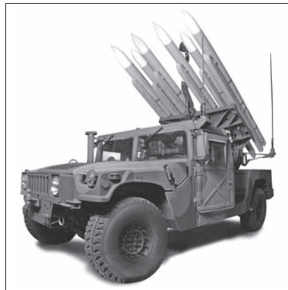
The futuristic Surface-Launched Advanced Medium-Range Air-to-Air Missile (SLAMRAAM) system gradually will replace the Avenger Air Defense system.
