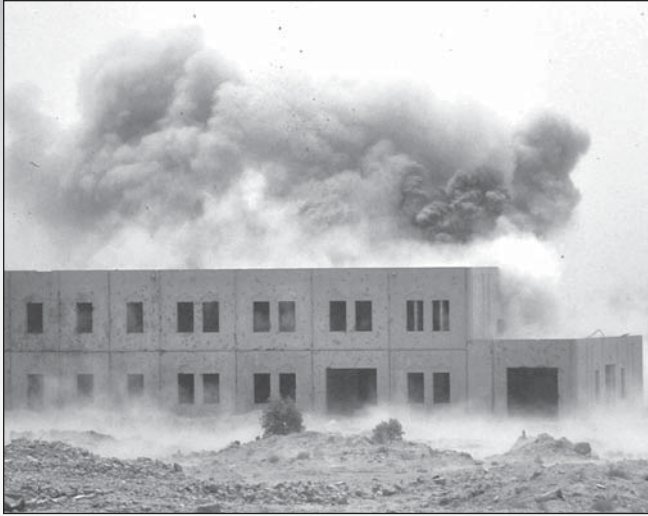
During testing in Iraq, GMLRS unitary hits the building on the far side, leaving the near side of the building intact.
