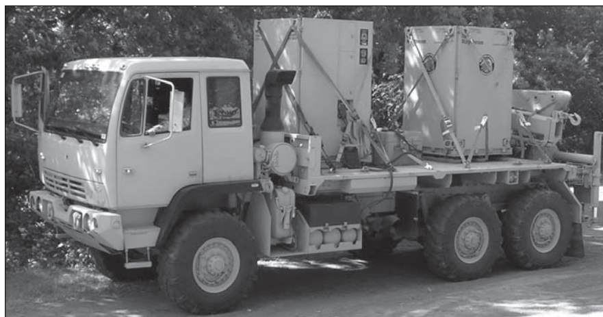
Family of Medium Tactical Vehicles (FMTV) Truck with two Non-Line-of-Sight Launch System (NLOS-LS) Container Launch Units (CLU) (Photo by Major (Retired) Mark Laflamme)
