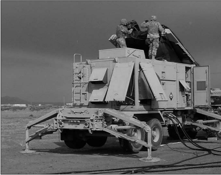
Two Soldiers from A Battery, 5th Battalion, 52nd Air Defense Artillery (A/5-52 ADA), uncover the Patriot Main Array Radar during crew drill training.
