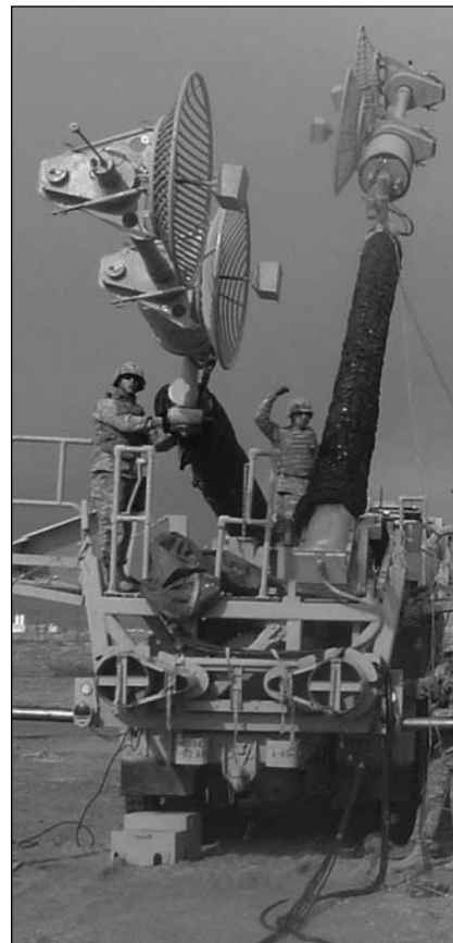
SPCs Eric Long (left) and Kevin Albers (center) with SGT Michael P. Bishop, all of A/5-52 ADA, set up the Patriot antenna mast group (AMG) during crew drill training.
