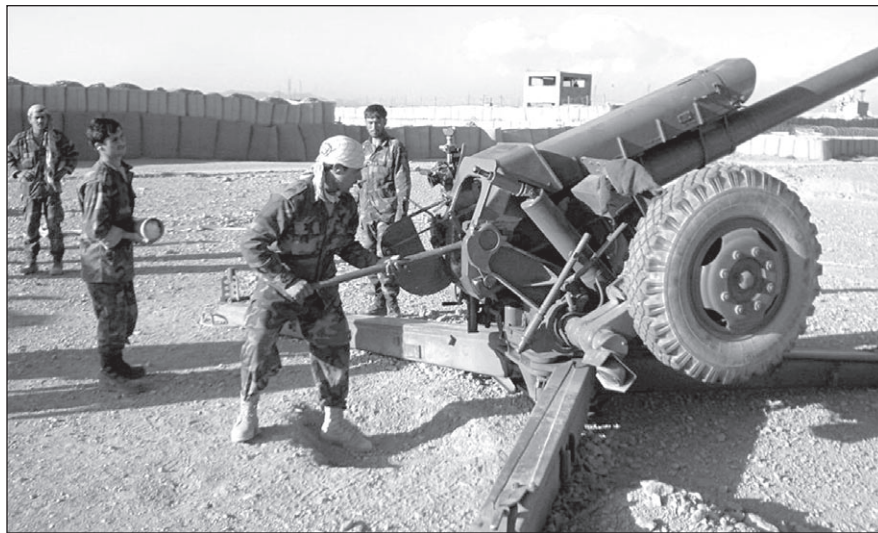
An Afghanistan National Army soldier rams the round into a Russian D-30 122-mm howitzer during training for the unit's first live fire. In October 2006, the 4th Battalion, 2nd Brigade, 203rd Corps Afghanistan National Army (4/2/203 ANA) FA battery became the first Afghan FA unit to shoot indirect fires in combat.
