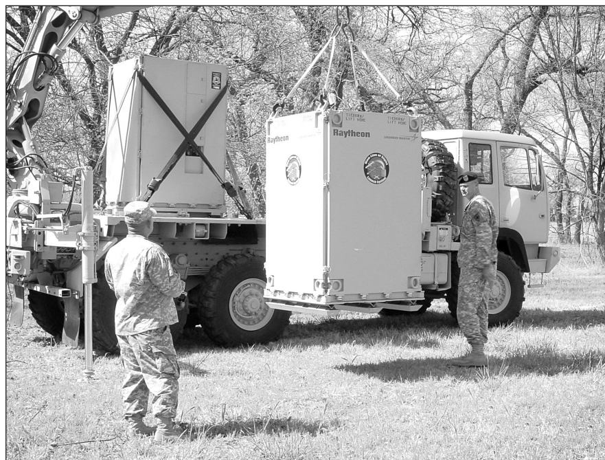
Soldiers train to download container launch units (CLUs). The CLUs can carry the precision attack missile (PAM), the loiter attack missile (LAM) or a mixture both.
