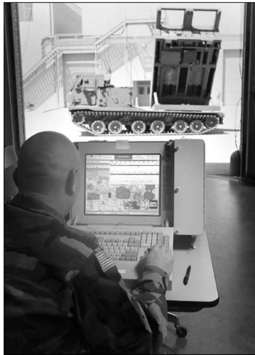
A 13P instructor for the New Equipment Training Division at the FA School sends fire missions to an M270A1 launcher using a battery AFATDS "box." Future users will be able to access AFATDS from their computers over the net concurrently with other applications.
