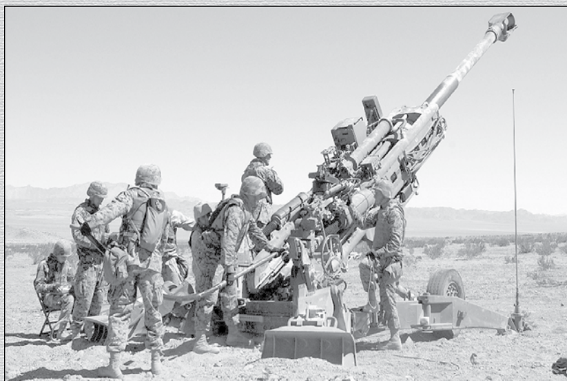
The lightweight 155-mm (LW155) joint towed howitzer eventually will replace all Marine Corps and Army M198 howitzers.
