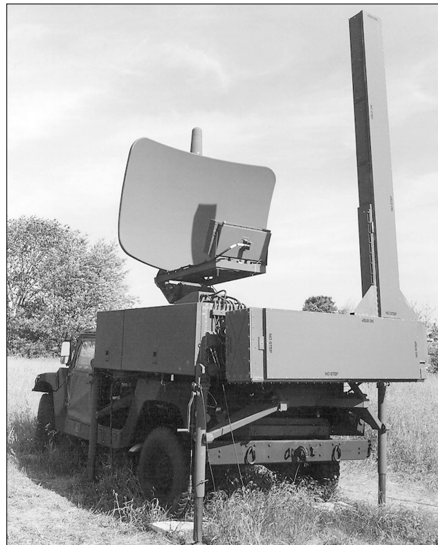
Army Aviation's Air Traffic Navigation, Integration and Coordination System (ATNAVICS). The multi-mission radar (MMR) will combine the capabilities of the Q-36, Q-37, Sentinel and ATNAVICS radars when the MMR is fielded in FY13.
