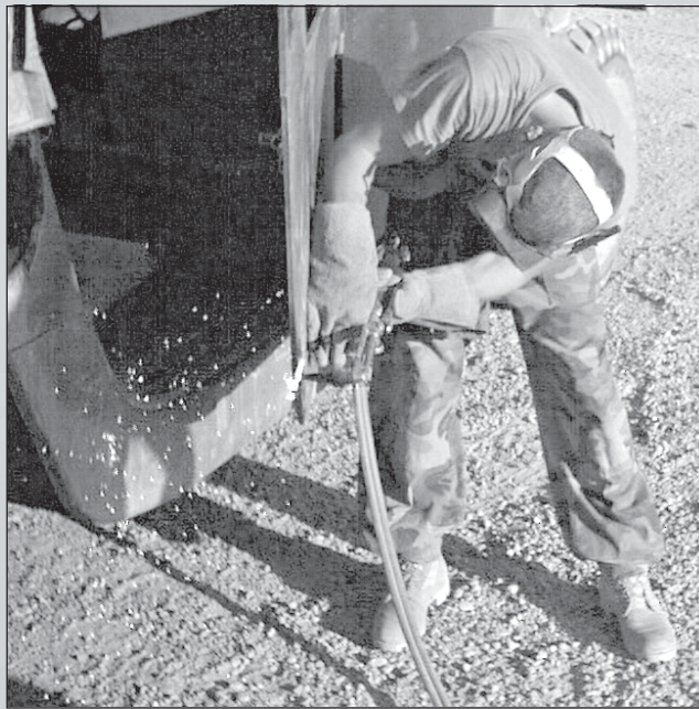
SGT John Blanshard welds armored doors onto a high-mobility multipurpose wheeled vehicle (HMMWV).
