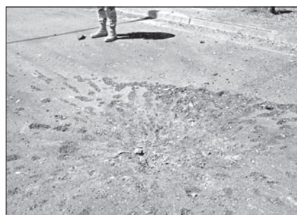
Although a 127-mm rocket impacted on concrete in Baghdad, (16 March 2005) the effects still are a good example of a high-angle rocket crater.
