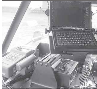
An MTS installed in a HEMTT.
