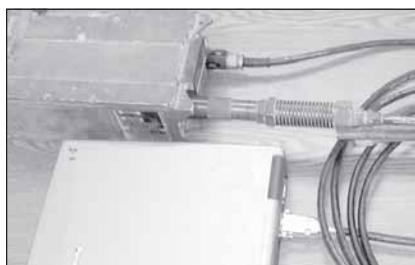
Figure 1: The digital cable links a single-channel ground and airborne radio system (SINGARS) to a laptop computer through the computer's serial port.
