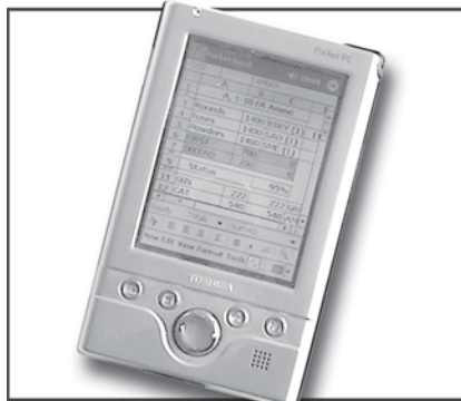
Figure 3: This is a personal digital assistant (PDA) showing a Microsoft Excel spreadsheet for use as an ammunition tracker.
