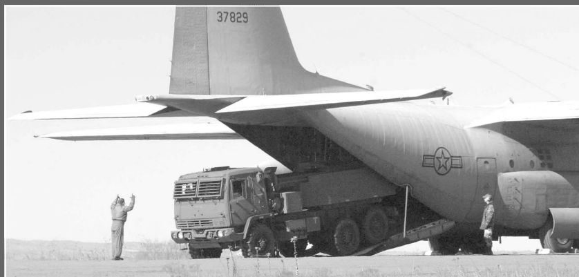
19 Nov 03, Fort Sill, OK—The high-mobility artillery rocket system (HIMARS) passes its C-130 Assault Landing Zone Test with “flying colors.” A combat-loaded HIMARS and three crewmen with combat gear were loaded into a C-130 at Redstone Arsenal, AL (a timed event); flown 660 nautical miles (the operational reach of Operation Iraqi Freedom) to an unimproved airstrip on Fort Sill’s East Range; exited the aircraft and recovered from air movement (a timed event); drove five kilometers rapidly to a firing point; and fired six reduced-range practice rockets (RRPRs)—demonstrating its deployability, mobility and lethality. (Photos by Fred W. Baker III, Fort Sill Cannoneer)
