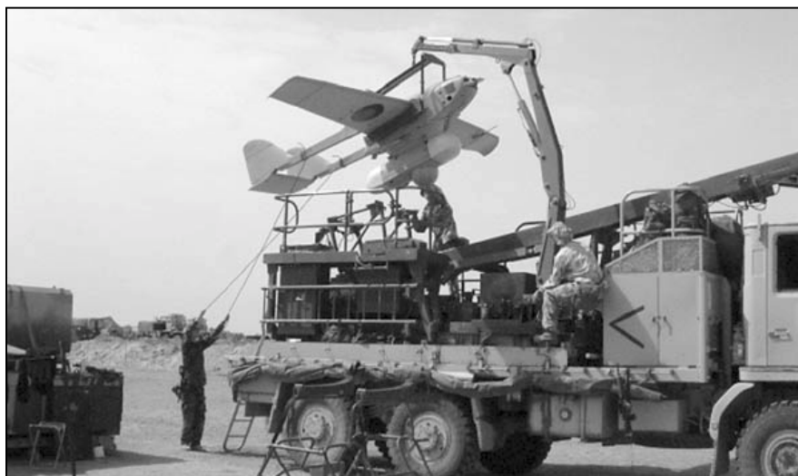
The British Phoenix unmanned aerial vehicle (UAV) being employed in Operation Telic. The Phoenix is rail-launched and operates from within the divisional area.
