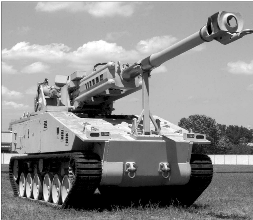
Non-Line-of-Sight (NLOS) Cannon. This approximately 20-ton demonstrator fired at Yuma Proving Ground in August. (Photo courtesy of United Defense)
