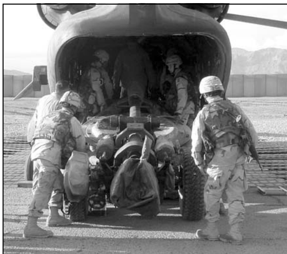
Internal loading allowed the Chinooks to be more maneuverable and move more quickly when they flew the howitzers to position areas and smaller firebases in the adjoining regions. In addition, this technique disguised the fact that a howitzer was being positioned on a firebase.
