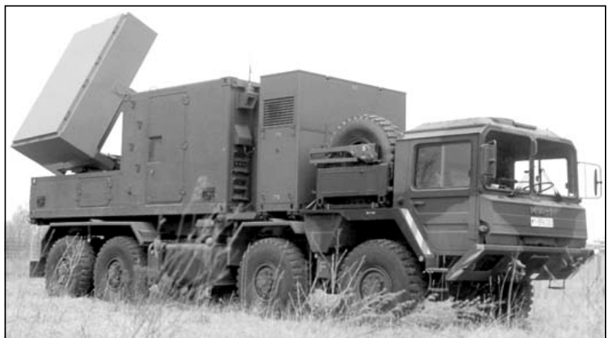
The Cobra counterbattery radar is a trilateral project: France, the United Kingdom and Germany
