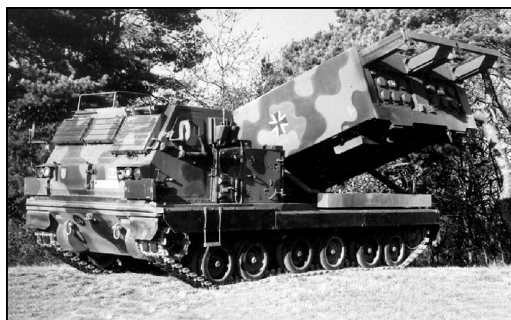
The medium artillery rocket system (MARS) is the same multiple-launch rocket system (MLRS) used in the US artillery.
