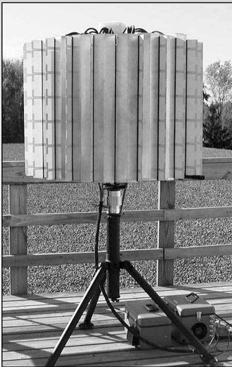
The lightweight counter-mortar radar (LCMR) developed by the Army's Special Operations community.
