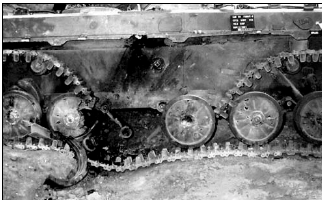
Figures 3: In a near hit, HE rounds with PD fuzes destroyed the track of this tank. The damage was similar to that of a tank in a hull-down position.
