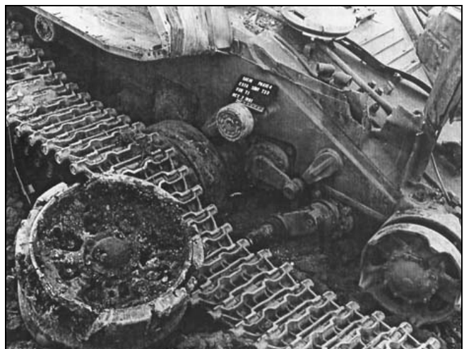
Figure 5: A 155-mm round impacted within 30 meters of this tank, causing considerable damage.
