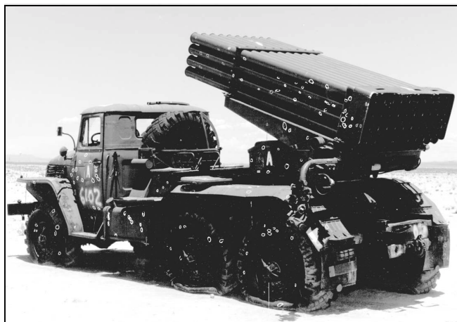
Figure 6: During testing, DPICM destroyed this multiple-rocket launcher (MRL). The MRL had no ammunition on board when it was destroyed; the destruction was due entirely to DPICM. The holes highlighted went through the entire vehicle.
