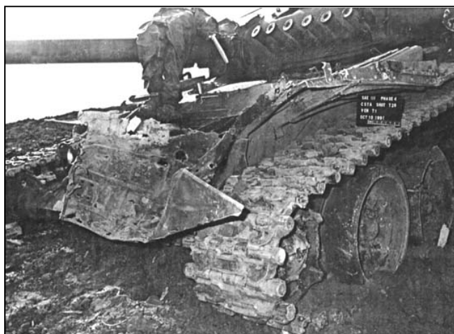
Figure 7: One round of HE with a PD fuze significantly damaged this tank in a near hit.
