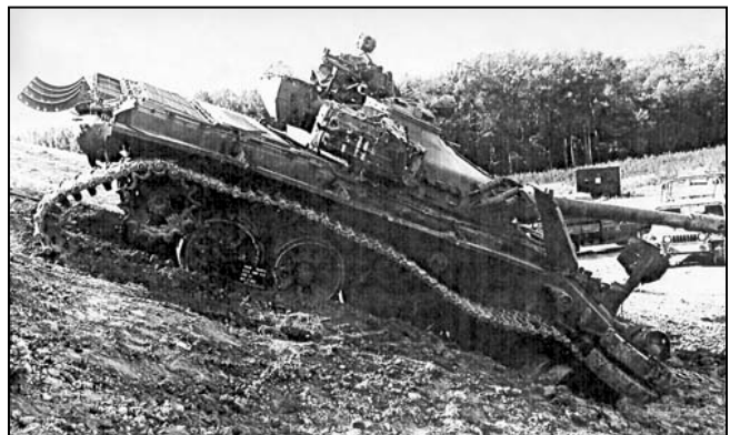
Figure 4: HE with PD in a near hit—the SAE tests confirmed the validity of the Soviet report showing artillery more lethal against armored targets than US effects estimates.
