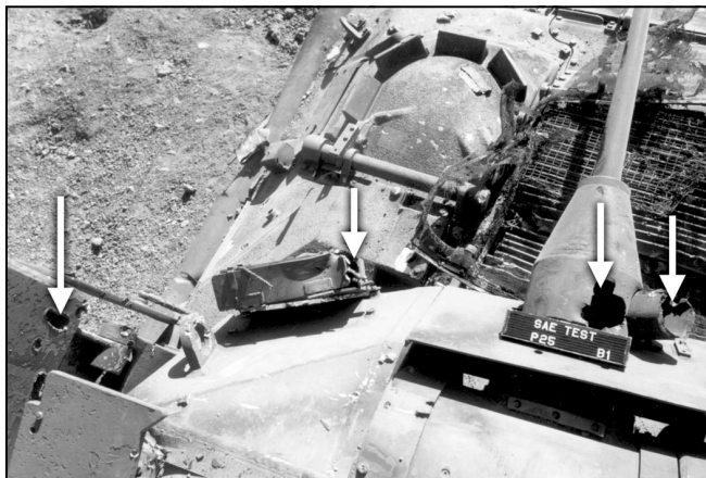
Figure 2: An air burst of HE with a variable time (VT) fuze destroyed the main gun and other components of this vehicle.
