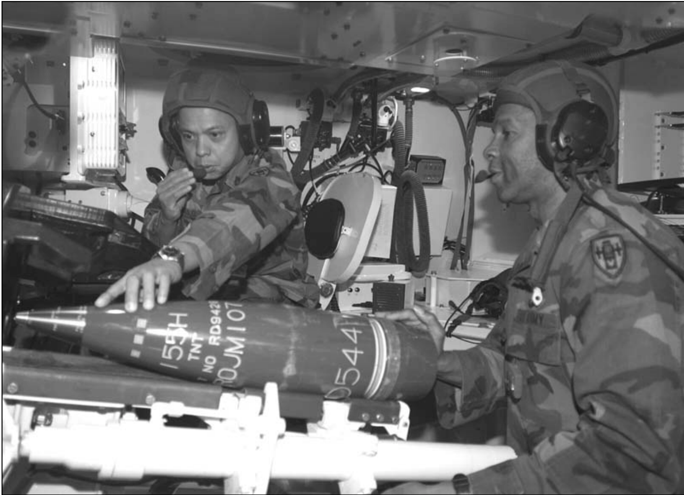
SSGs Restituto Carrillo and Neville Abram, L-R, Gunnery Department instructors, verify the fuze type and setting before loading a projectile into the new Paladin Fire Support Combined Arms Tactical Trainer (FSCATT). Photo by Fred W. Baker II, Fort Sill Cannoneer.
