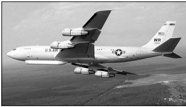
USAF E-8 Joint Surveillance and Target Attack Radar System (JSTARS). This aircraft is a long-range air-to-ground surveillance platform designed to locate, classify and track ground targets.
