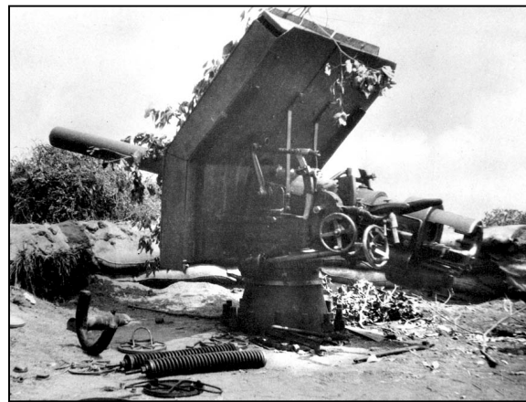
A 105-mm gun from the Königsberg mounted on a static carriage for the defence of Mwanza. (Courtesy of the Imperial War Museum, London)
