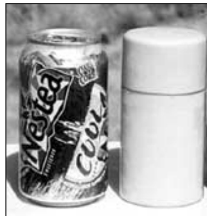
This one-watt jammer disguised in a soda can has an effective range of 20 to 40 nautical miles.
