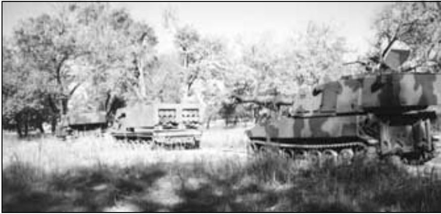
The Second (and Latest) Revolution in American Artillery—the M270 MLRS and the M109A6 Paladin. Computer and communications technology combined to enable these weapons to operate virtually autonomously anywhere on the battlefield, ideal for a Battery Team.
