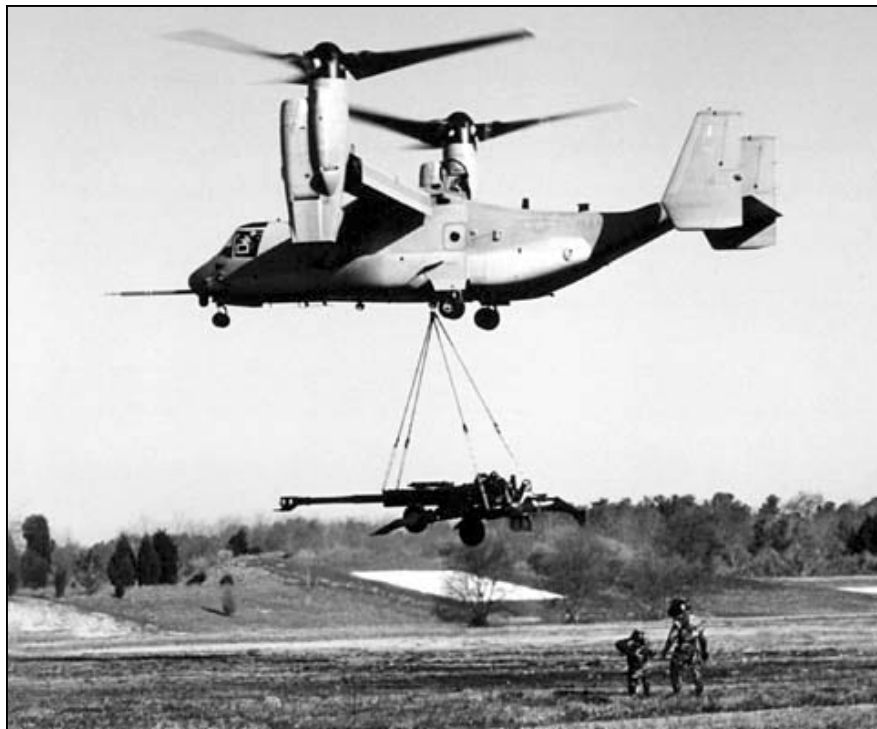
A Marine Corps MV-22 Osprey prepares to deliver an M777 lightweight 155-mm howitzer.
