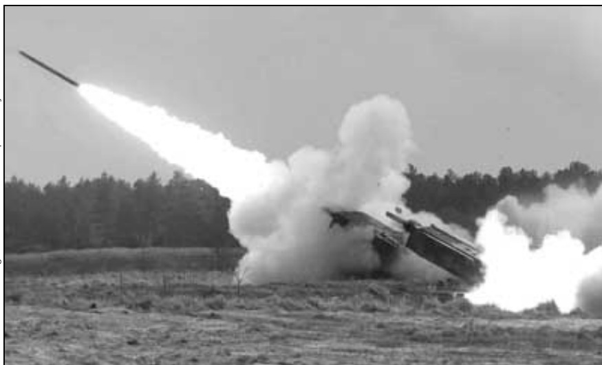
HIMARS is uniquely capable of supporting strategic early entry or contingency force operations because it can be deployed by C-5B, C-17 or intra-theater by C-130 cargo aircraft.
