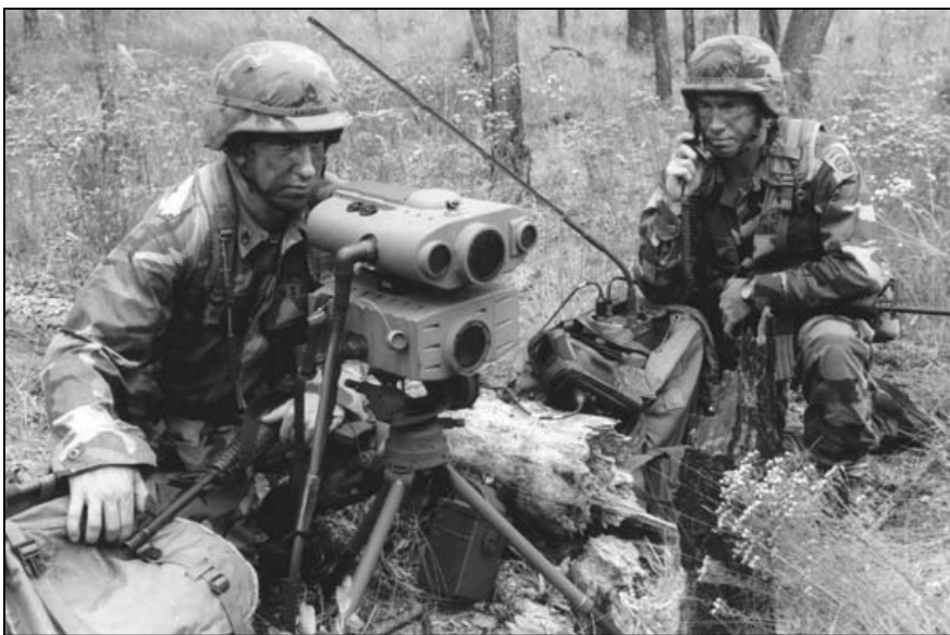
The lightweight laser designator rangefinder (LLDR) will weigh 35 pounds, including a day sight with ranges out to 10 kilometers, a thermal night sight with ranges out to two kilometers, a laser rangefinder, laser designator and tripod. (Photo Courtesy of Litton Laser Systems)
