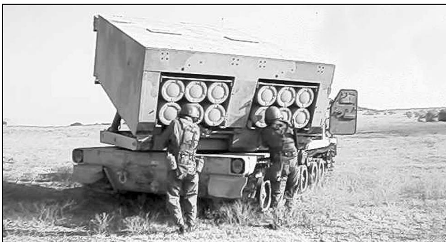
Standard reload time from ammunition already on the ground near the firing position is 20 minutes. If the ammo is not already on the ground, this process can take an hour or more, significantly longer than the minute it takes to select a different shell/fuse combination for Paladin.
