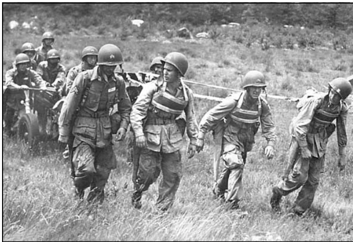
1943 photo showing a pack howitzer crew moving the gun with a system on harnesses. These harness assemblies went in the paracrates and were dropped with the gun.
