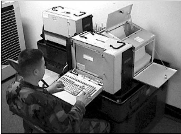
This FSTDS operator is working a multi-workstation operational facility (OPFAC) that also shares a hardened printer for both FSTDS systems.
