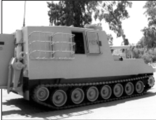
The Egyptian Army's 122-mm self-propelled gun is a combination of the Russian-designed, Egyptian-built 122-mm D-30 towed howitzer and our M109 chassis/drive train.
