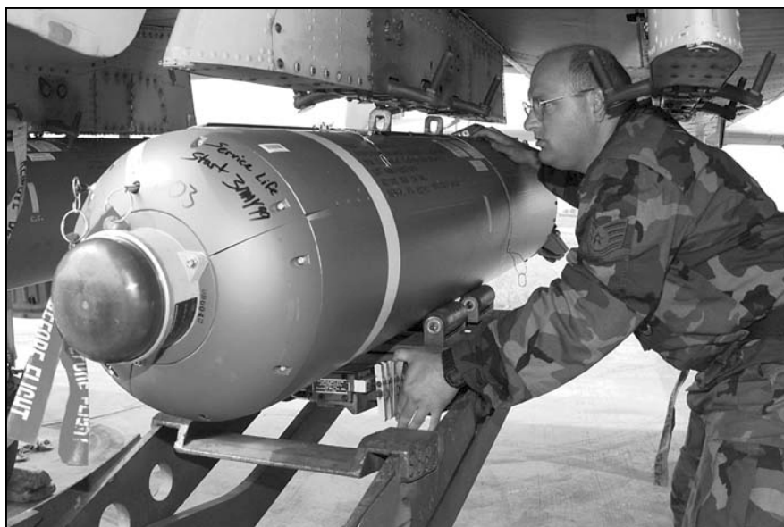
An ammo handler prepares to load a CBU-87 bomb on to an A-10 before the use of cluster bombs were restricted in Operation Allied Force.
