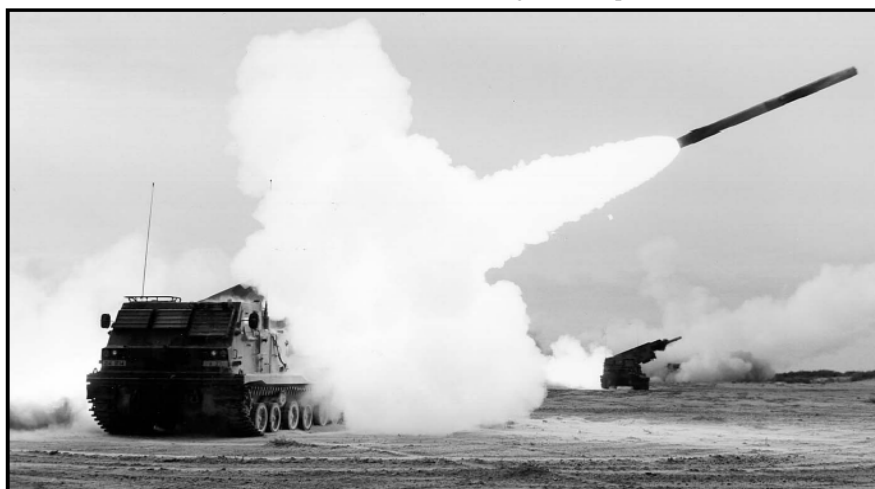
The extended-range MLRS (ER-MLRS), already in production, will fire out to 45 kilometers while the guided MLRS (GMLRS) improves accuracy and extends our range to 60 kilometers.
