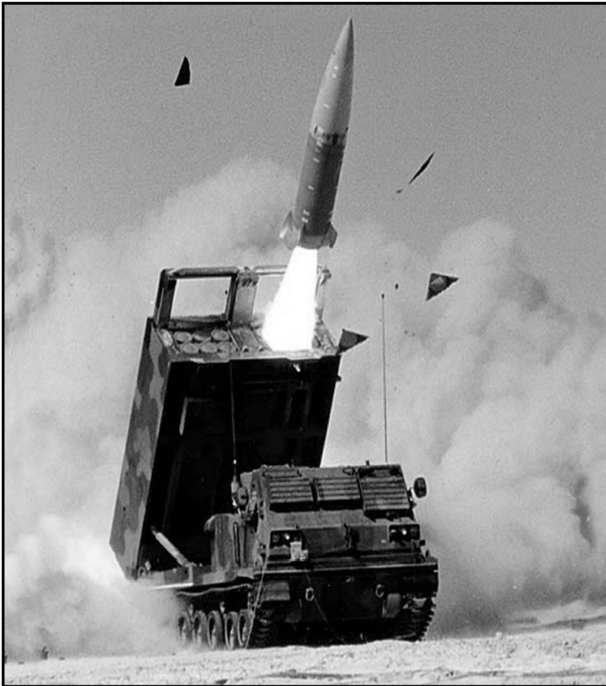
ATACMS fires-Block IA that reaches out 300 kilometers is fielding now. CENTCOM is developing a guide for controlling and integrating land and air fires for forces in its AOR.
