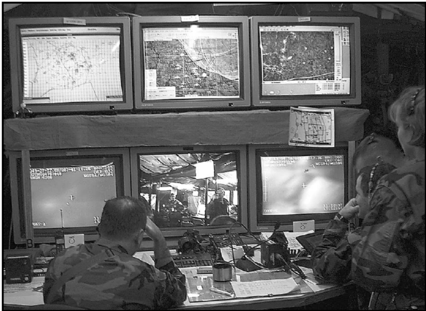
The DTAC's Deep Cell. From the Top, Left to Right: the Advanced Field Artillery Tactical Data System (AFATDS), friendly picture in the Maneuver Control System/Phoenix (MCS/P), enemy picture in the All-Source Analysis System (ASAS), the sensory picture of an unmanned aerial vehicle (UAV), a monitor with a video teleconference and one with another UAV picture.
