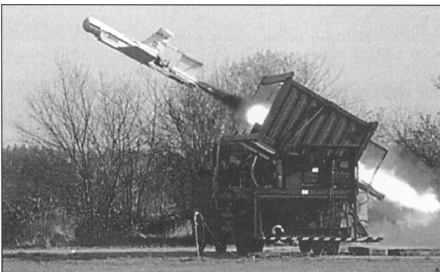
The CL 289 Reconnaissance Drone system has a range of 400 kilometers and can transmit infrared (IR) sensor data in near real-time out to a range of 75 kilometers and take IR and black-and-white pictures.
