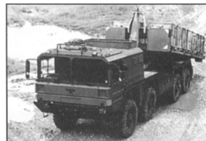
Multi is a 14-ton multipurpose resupply vehicle with a palletized loading system; the German Field Artillery will start fielding its Multi for ammunition resupply in 1999.
