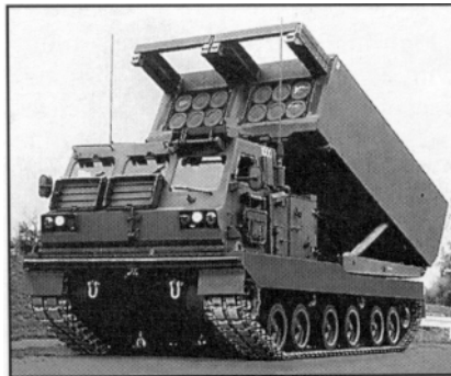
Shown here is the medium artillery rocket system ( MARS ), the US-made multiple-launch rocket system ( MLRS ).
