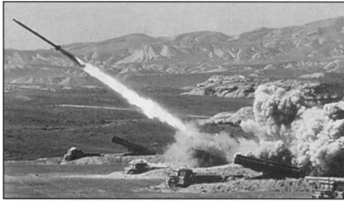
Built in 1974, the Uragan multiple rocket launcher (MRL) was designed to destroy targets up to 35 kilometers away.
