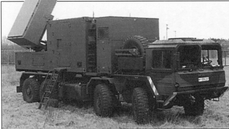
The Cobra counterbattery radar, a joint development by Germany, France and the United Kingdom, is still undergoing trilateral troop trials. Using state-of-the-art radar technology, this system tracks up to 40 trajectories in two minutes and determines the firing positions.
