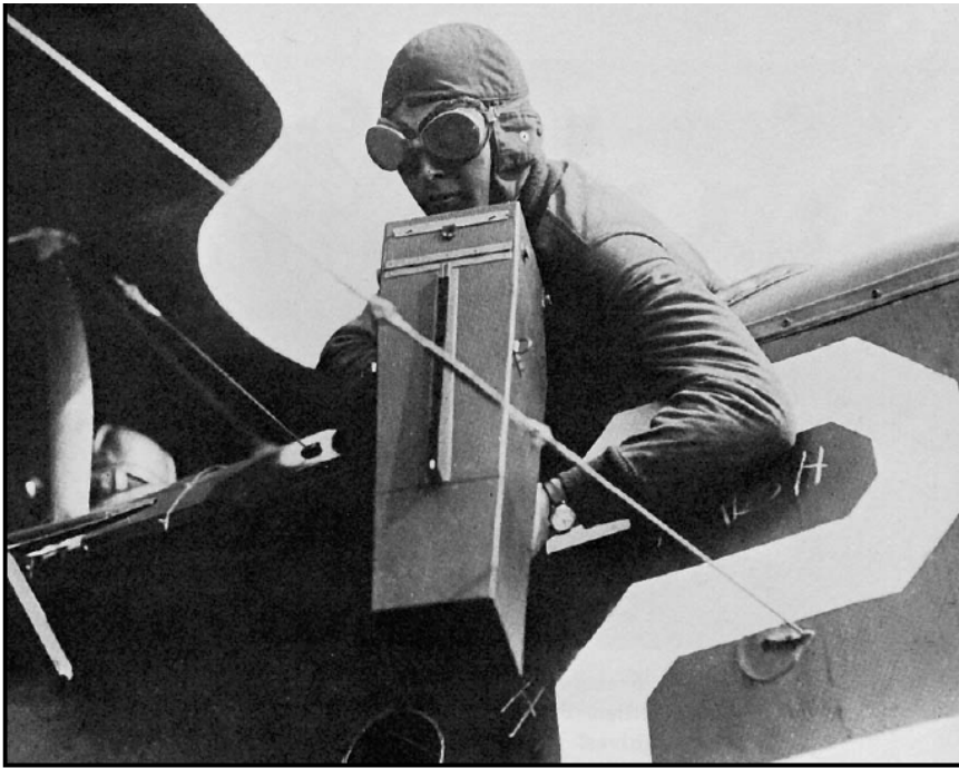
Aerial photography permitted precise targeting throughout the theatre and up-to-date mapping of ever-changing trenches. Here an observer operates the Graflex camera from an observaton plane.
