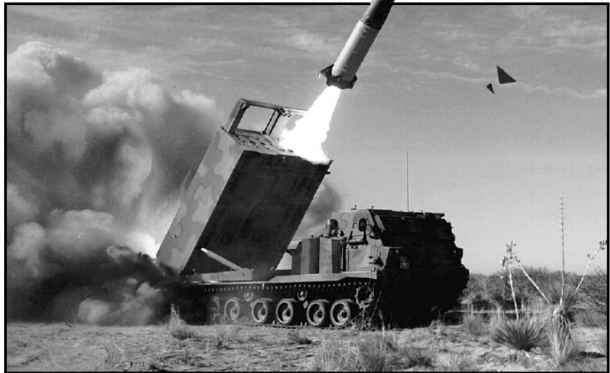
US Army Tactical Missile System (ATACMS). By 2005, ATACMS Block IIA will be able to prosecute the deep attack out to 300 kilometers.
