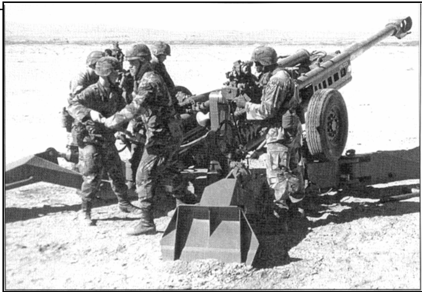
The new LW155 weighs nearly half of our current 155-mm towed howitzer and fires twice as fast, significantly increasing the lethality of our Army light and Marine forces.
