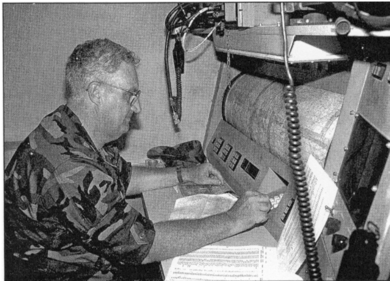
CW2 James Horn, F/109 FA (TA), acquiring targets inside the AN/TPQ-36 Firefinder radar shelter. (Photo by MAJ Peter Grzywacz)
