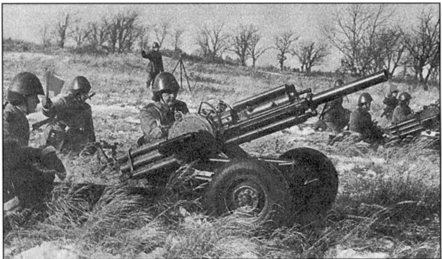
Mortars (part of Soviet artillery) often were attached to maneuver companies. The 82-mm Vasilek automatic mortar batteries (shown here) provide both indirect and direct fire and were particularly welcome by maneuver units.
