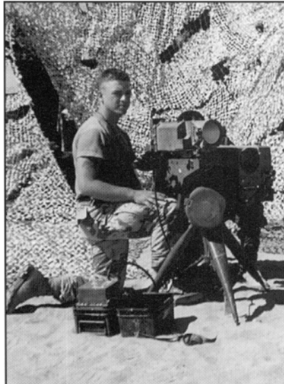
SGT Kirchoffer with the FIST's ground/vehicular laser locator designator (G/VLLD) in Kuwait.
