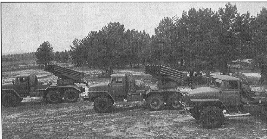
The Soviets often used the unarmored BM-21 MRL when other direct fire failed to dislodge the enemy. The truck-mounted BM-21s usually were moved into direct firing positions under the protection of an air strike, and each fired its 40 122-mm rockets immediately after the air strike ended.
