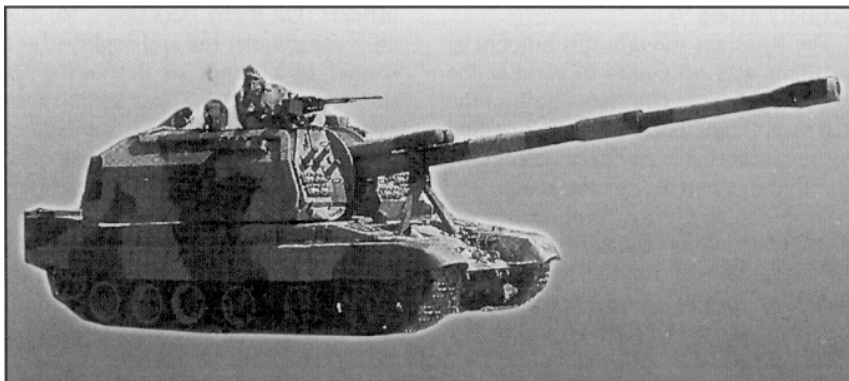
The 2S19 MSTA 152-mm self-propelled howitzer is a highly accurate weapon that can fire laser-guided munitions such as the Krasnapol projectile.
