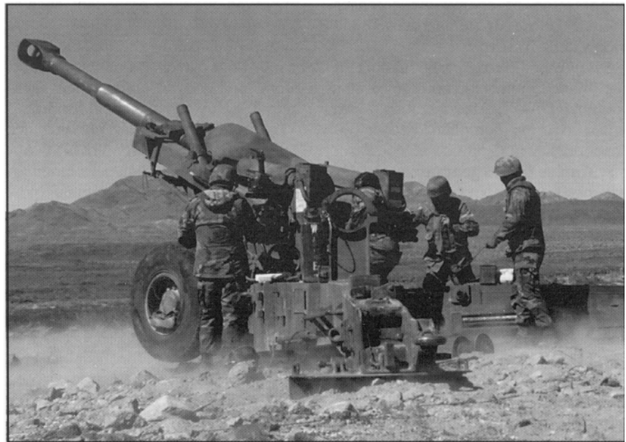
The M198 is much criticized for its weight and size. Its maximum range of 30 kilometers is significantly less than the ranges of many threat artillery systems.
