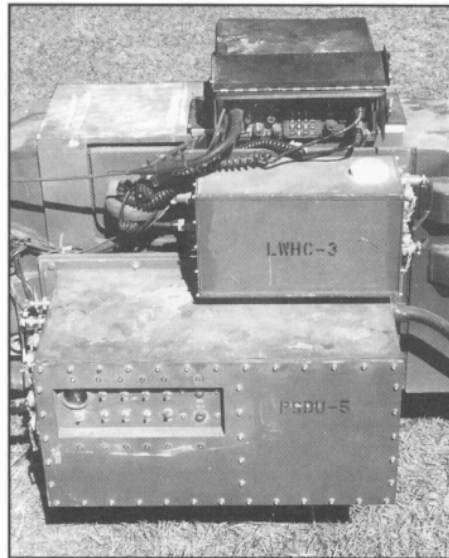
Howitzer: (from top to bottom) SINCGARS radio, on-board ballistic computer/radio interface and power supply.
