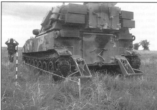
A 13B10 student is backing the 155-mm howitzer in position to lay on the the aiming circle at Fort Riley. The howitzer is positioned on the gun guide stakes.
