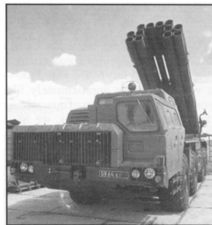
The Smerch 300-mm Multiple-Launch Rocket System. Smerch fires 12 rockets from 20 to 70 kilometers.
