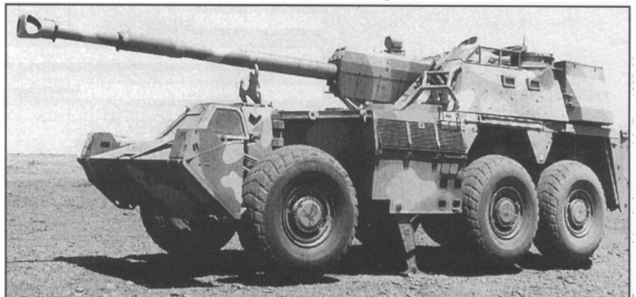
This South African G-6155-mm self-propelled gun-howitzer has its stabilizers lowered for firing.
