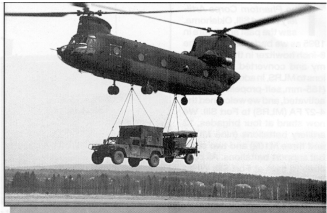
A/25 FA sling loads a Q-36 radar coupled with its prime mover.
