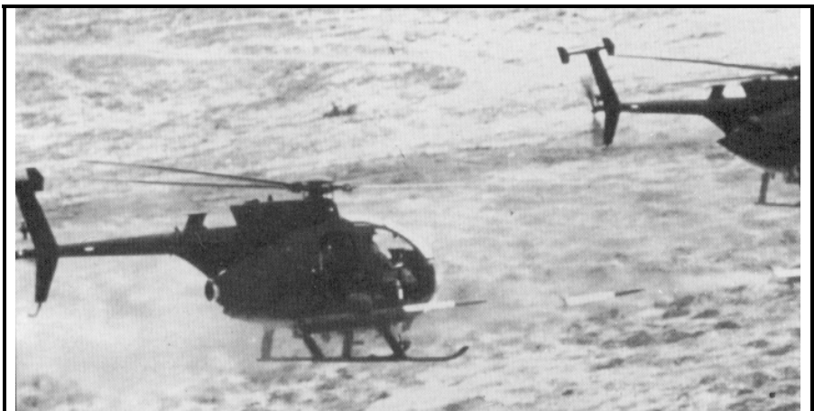
AH-6 Cayuse helicopters fire 2.75-inch fin-folding rockets. The Cayuse is a key fire support platform for multiple special operations.
