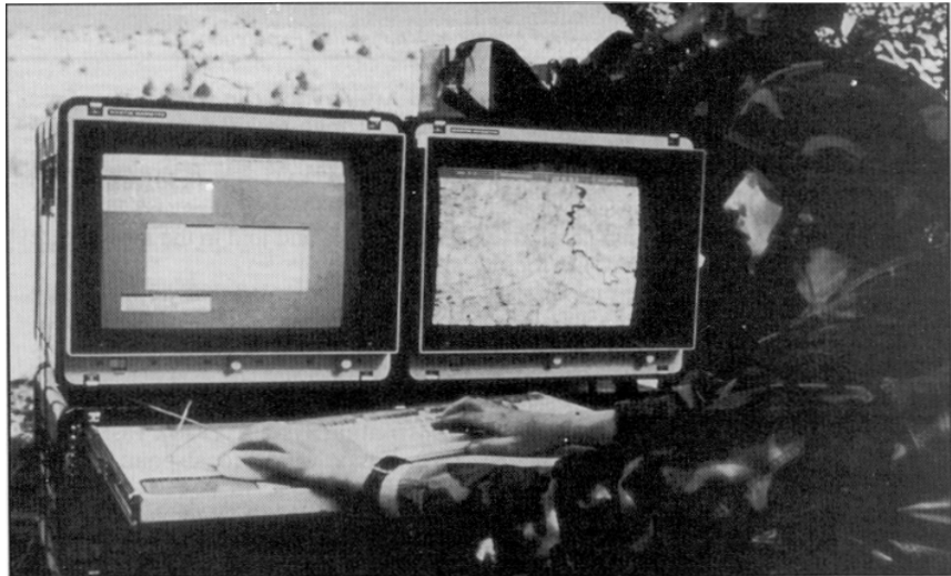
ASAS is the intelligence electronic warfare (IEW) subelement of the Army tactical command and control system (ATCCS). It gives combat leaders battlefield intelligence from joint strategic and tactical sensors.
