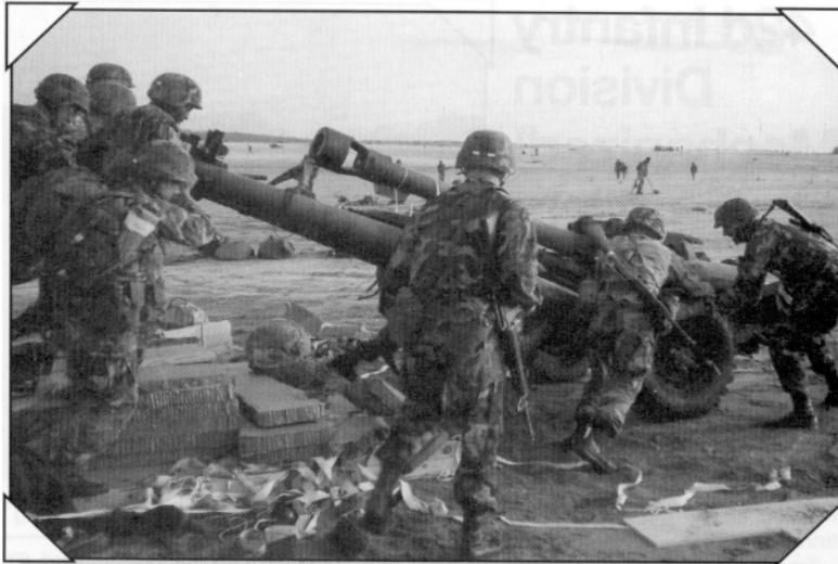
A howitzer is de-rigged and all troopers "stand-in" to get the piece off the platform.
