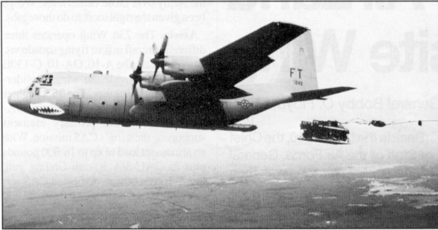
A Pope AFB C-130 Hercules heavy equipment load exits the aircraft during a practice supply delivery. The C-130's container delivery system uses gravity to pull from one to 16 bundles of supplies from the aircraft.
