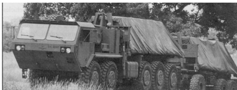
The 10x10 axle design (all five axles drive) provides excellent weight distribution between the axles to increase off-road mobility.
