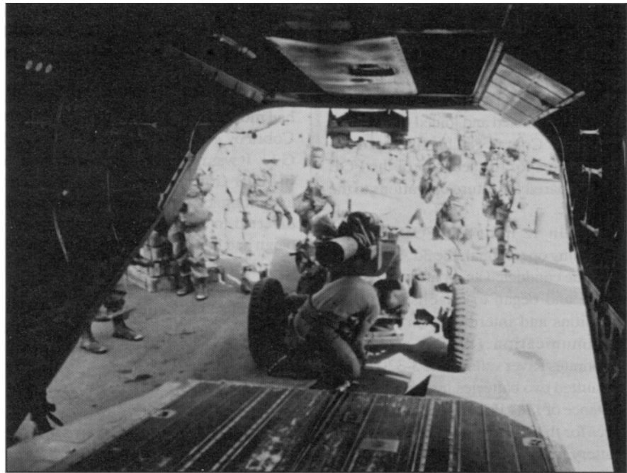
Using CH-47 helicopters as the 105-mm howitzers' prime movers, the 101st Airborne Div Arty trained for extended air assault artillery raids.
