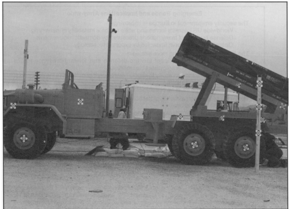
Preliminary Testing for HIMARS Development. In April at White Sands Missile Range, New Mexico, this modified Honest John missile launcher successfully fired multiple launch rocket system (MLRS) rockets in a test to see if rockets could be fired from a vehicle.
