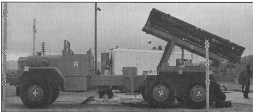
HIMARS Testing. In April, the Field Artillery School tested the HIMARS concept by launching MLRS rockets from a truck bed at White Sands Missile Range, New Mexico.
