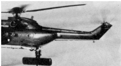
Orchidee Radar Mounted under a Helicopter
