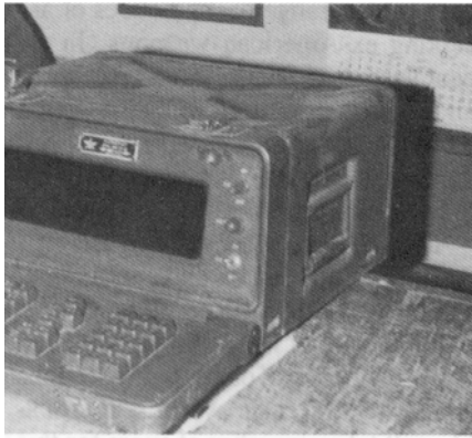
This ROKA fire direction computer is used at the battery and battalion levels.
