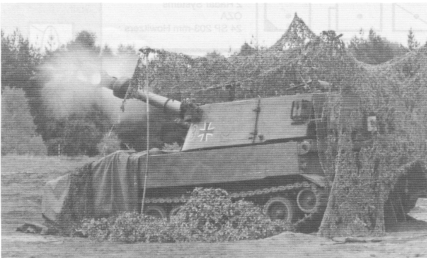
This M109 howitzer will be in service well beyond the year 2000. We've increased the range to 24 kms (30 kms firing base bleed) and will retrofit it with the AURORA navigation system.
