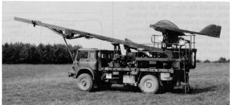
The Phoenix RPV provides real-time surveillance and target acquisition thermal imagery far beyond the FEBA.
