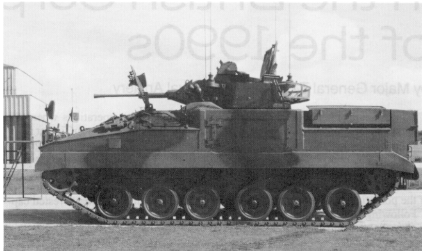
This FOO's variant of the Warrior mechanized infantry fighting vehicle has observation and target acquisition devices mounted under armour.
