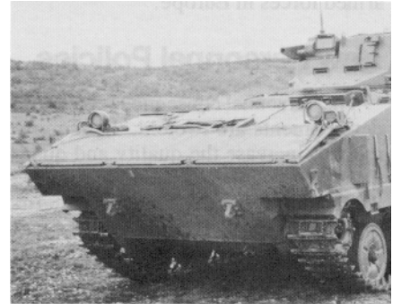
The VOA, currently being fielded in Field Artillery batteries, has a laser range finder, thermal camera and digital message device.
