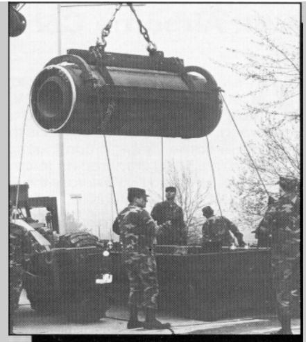
Soldiers of 4-9 FA lower the second stage of a PII missile into a storage container.
