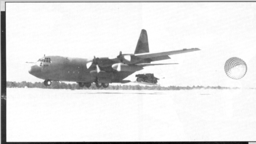
The low-altitude parachute extraction system (LAPES) is another way to get the Contingency Corps' equipment on the battlefield rapidly.
