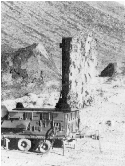
A 5th Infantry Division AN/TPQ-37 Firefinder Radar. Larger and more powerful than the AN/TPQ-36, the Q-37 can locate enemy cannons and rockets at ranges of 50 kilometers.
