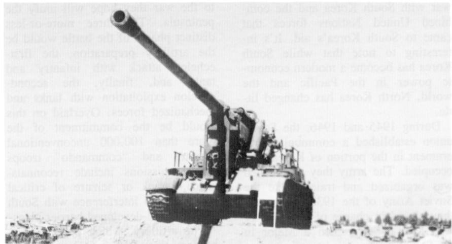
The 170-mm self-propelled gun is uniquely North Korean and has the longest range of any cannon in any army—an estimated 50,000 meters.
