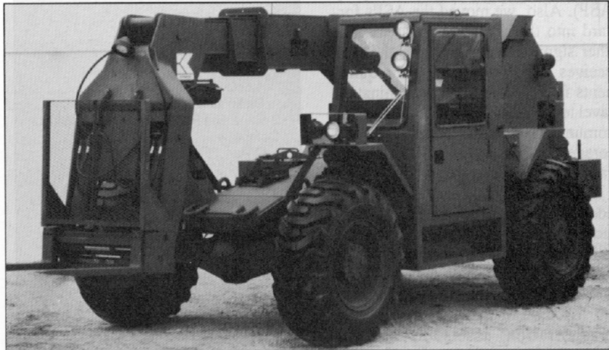
The 6,000-Pound Variable-Reach Rough-Terrain Forklift
