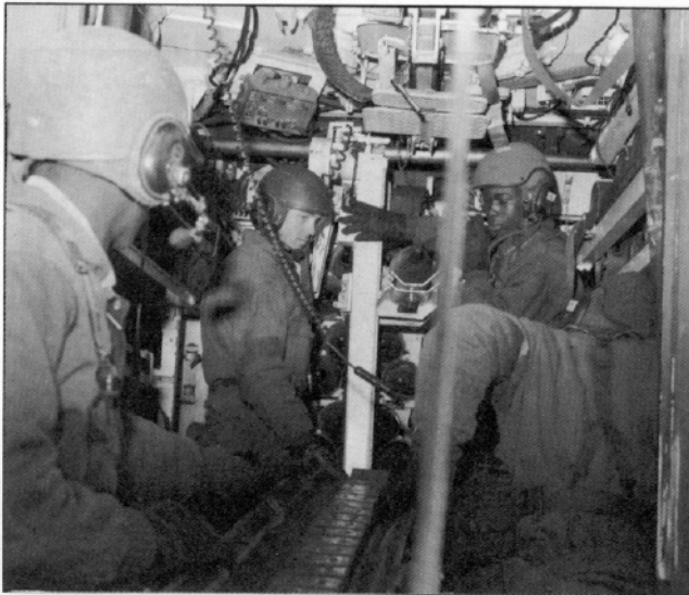
Soldiers of A Battery move rounds onto the conveyer belt in the FAASV.
