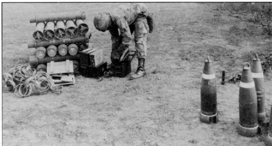
Preparing a Howitzer or Field Artillery Ammunition Support Vehicle (FAASV) Rearm Cache
